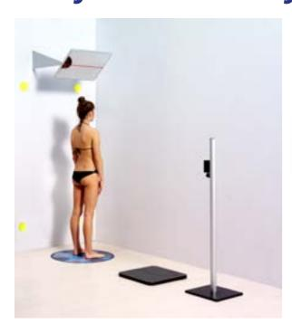
The system is composed of a camera with its support, mirror and fastening clamps, colored discs for the location referencing of the pictures and an adhesive screen-printed disc to be placed on the ground for the positioning of the patient.
