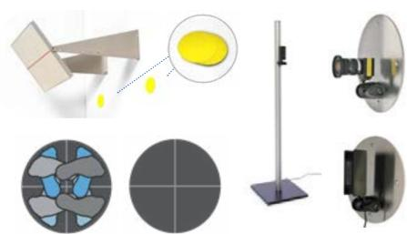
**PHYSICAL ANALYZER** is a device for the postural analysis of a patient on the frontal/rear and lateral plane. It is innovative for the positioning on the wall of the colored disks and the location referencing of the pictures. The aluminum cage and the lead string are no longer necessary reducing the space required. The software, recognizing the position of the four yellow disks on the wall, determines the vertical
