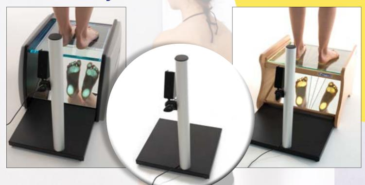
FOOT ANALYZER: Multi-purpose device equipped with a wooden platform, camera and support to acquire images of the podalic load and the rear foot. The software that allows the management of the images (the same one that manages the photos of the body and the stabilometric analysis) is perfect for those who want to save the images of their patients for a correct evaluation over time.
